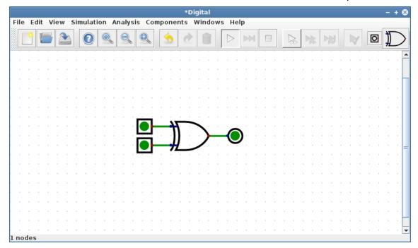
Interaction with the circuit is possible when simulation is started. This is done by clicking on the play button located in the toolbar. After starting the simulation, the color of the wires changes and the inputs and outputs are now filled. Bright green indicates a logical '1' and dark green a logical '0'. In the figure above, all wires have a '0' value.
