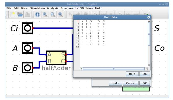
In order to check the correct function of the full adder, a test case should be added. In the test case, the truth table is stored, which should fulfill the circuit. In this way it can be automatically checked whether this is the case.
