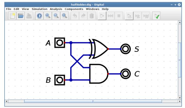
As an example, consider a 4-bit adder: First, we built a simple half-adder. This consists of an XOR gate and an AND gate. The sum of the two bits 'A' and 'B' is given to the outputs 'S' and 'C'. This circuit is stored in the file *halfAdder.dig*.
