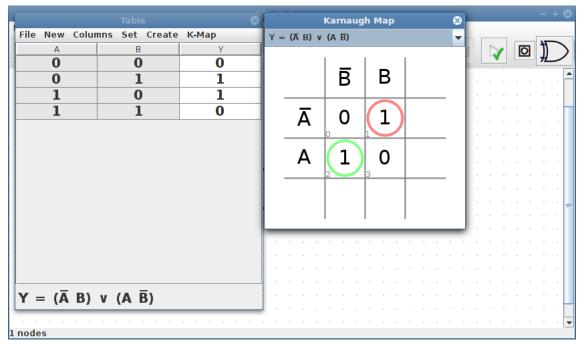
At the top of this dialog there is a drop-down list which allows the selection of the desired expression in the K-map. In this way you can, for example, illustrate how several equivalent algebraic expressions can result. However, in this example, there is only one minimal expression. The truth table can also be modified by clicking the K-map.
