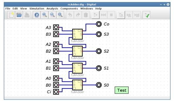
Now the full adders can be put together to form a so-called ripple-carry adder. In this case, the carry output of an addition is forwarded as a carry input to the addition of the next higher-order bit, just as is usual in pencil-and-paper addition. This 4-bit adder should be tested for correct function. For this purpose a test case was inserted.
