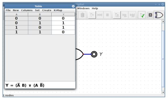
The truth table of the simulated circuit appears in a new window. Below the table you can find the algebraic expression associated with the circuit. If there are several possible algebraic expressions, a separate window will open, showing all possible expressions.
