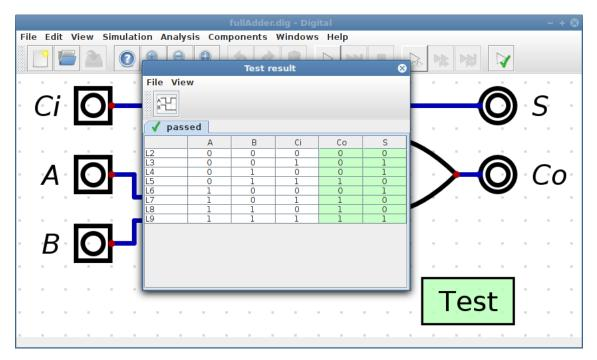
The tests can be executed via the test case editor or the test button in the toolbar. The table cells highlighted in green indicate that the output of the circuit matches the truth table given in the test case.
